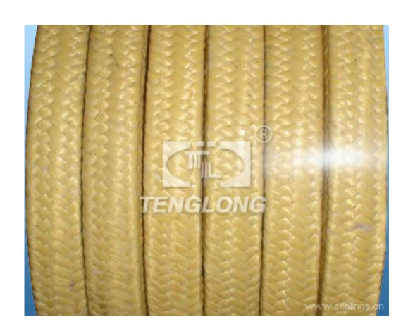
Description:STYLE 6500 Aramid fiber braided packing is made of Du Pont's continuous filament Kevlar yarn impregnated with PTFE emulsion and processed with lubricant. As the strength and module of Kevlar is as high as the steel-like strength, it can resist more serve media and higher pressure. It can be installed separately or as end rings with other kinds of packing to combine different characteristics into seals packing ring set.
